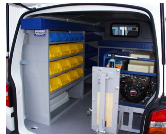
Standard interior racking solution with custom-built equipment and power supply
