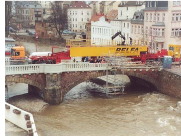
BELFA, semitrailer for testing the safety of bridges with a total gross weight of more than 100 t
