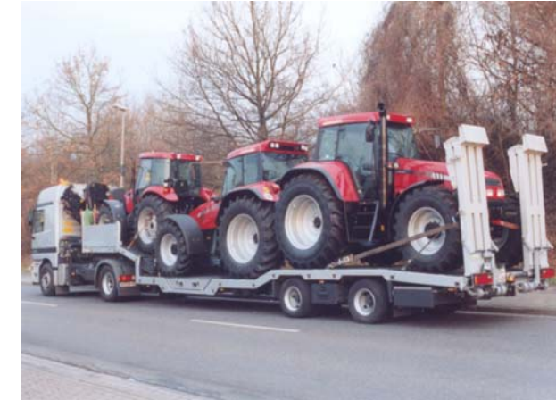
Specially built semitrailer for the transport of heavy tractors
